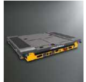
The UPC Shuttle (Under Pallet Carrier) travels independently underneath the stored pallets.
