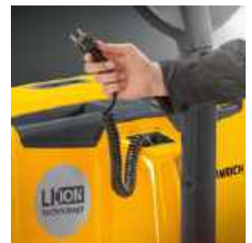
Easy intermediate charging thanks to on-board charger.
