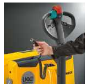
Intermediate charging at any socket: The integrated charger.
